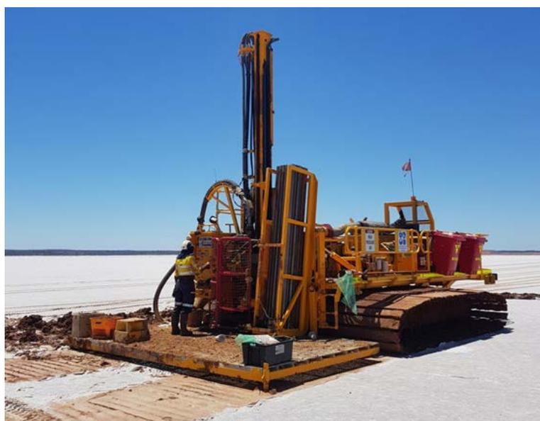
Figure 1 AC Drill rig underway on Lake Lefroy (Photo courtesy of Gold Fields)
